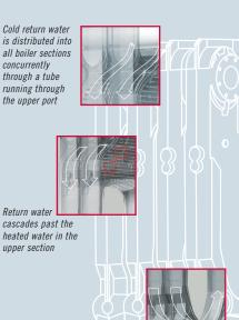
As heated water circulates through the main section, it offsets thermal shock caused by the introduction of cold return water
